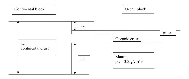
2. Write a program that instantaneously removes (erodes) 1 km of crust from the top of the 40 km continental crust. The continental crust is now 39 km thick. Recalculate the elevation of the continental crust with respect to mean sea level  $(T_e)$ . How many meters did isostatic re-equilibration cause the top of the 39 km thick crust to go up or down AFTER the erosion event?
